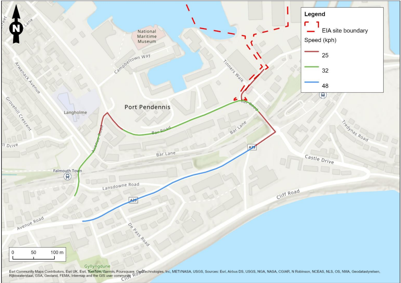
Figure A15.2.1: Modelled Road Network and Road Link Speed for Demolition and Construction Scenarios
